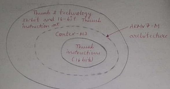
Fig 1: Relationship between the Thumb Instruction Set in Thumb-2 Technology and the Traditional Thumb.
