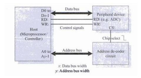
A **parallel port** is a type of interface found on computers (personal and otherwise) for connecting peripherals. The name refers to the waythe data is sent; parallel ports send multiple bits of data at once, in parallel communication, as opposed to serial interfaces that send bits one at a time. To do this, parallel ports require multiple data lines in their cables and port connectors, and tend to be larger than contemporary serial ports which only require one data line.
