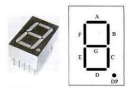
A seven-segment display (SSD), or seven-segment indicator, is a form of electronic display device for displaying decimal numerals that is an alternative to the more complex dot matrix displays. Seven-segment displays are widely used in digital clocks, electronic meters, basic calculators, and other electronic devices that display numerical information.
